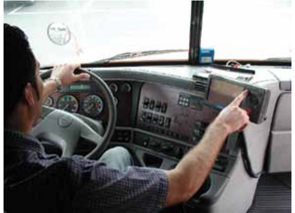
Schneider National is implementing Maptuit NaviGo on its Qualcomm MCP200 in-cab computers.
